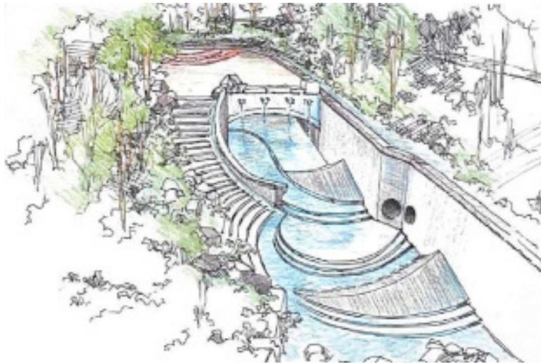
ABOVE The Re-evaluating Stormwater Plan (1998) redesigned the Nine Mile Run outflow to dissipate the water's energy as it exited the culvert and to provide safe access to the stream for park visitors.
